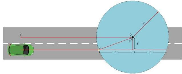
Fig. 4 Distance between the vehicle and RSU range
