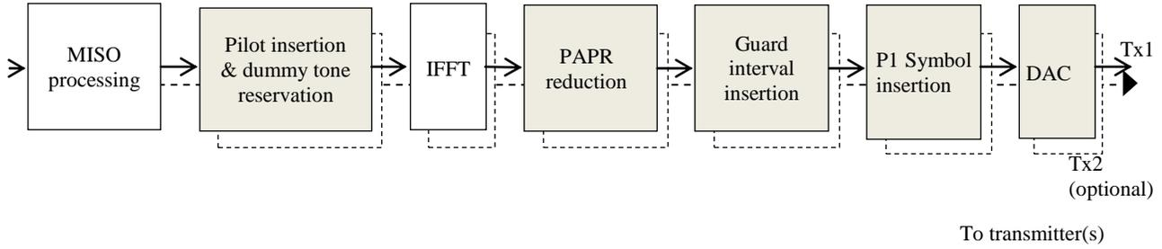
Fig. 1 The front end of the DVB-T2 transmitter [33]
