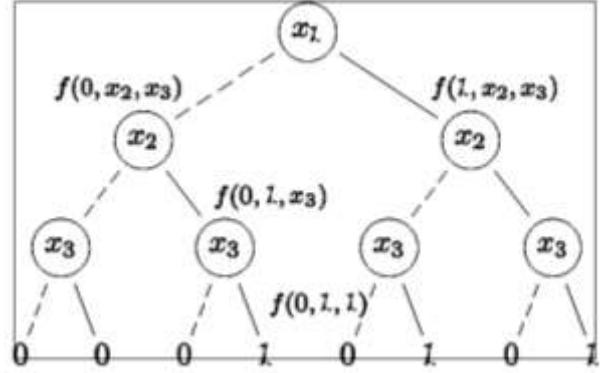
Fig. 1. A completely unreduced BDD which represents the Boolean function  $f = \neg x_1 \cdot x_2 \cdot x_3 + x_1 \cdot \neg x_2 \cdot x_3 + x_1 \cdot x_2 \cdot x_3$ .
