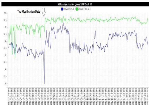
Figure 11. Quality stability after enabling the self-optimization model
